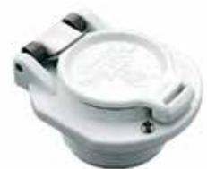
For pools with a dedicated suction line, Hayward recommends the Vac Lock™. It's a safety mechanism with a spring action cover, to hold the hose and close the suction opening when not in use.
